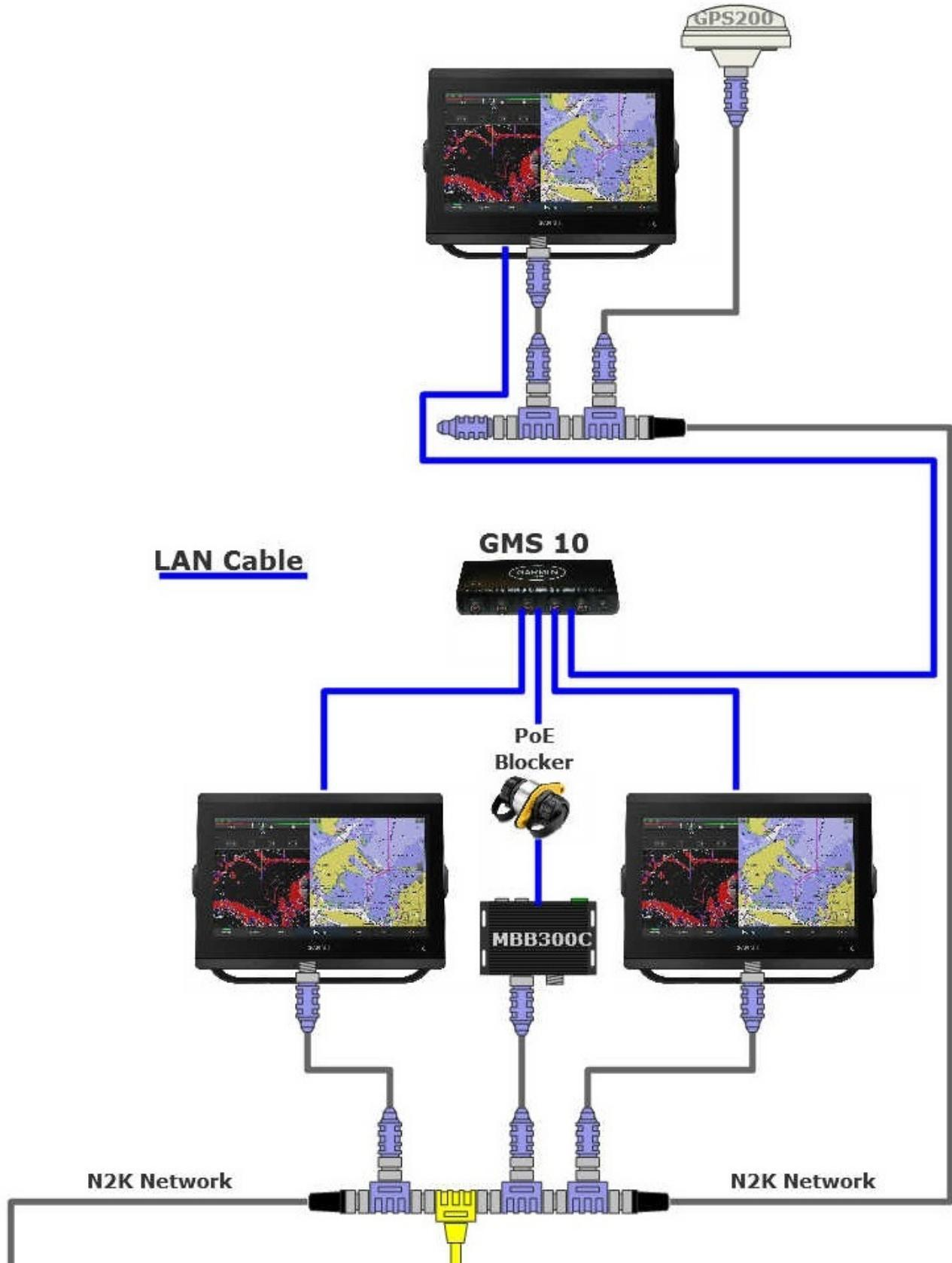
Once you Maretron MBB300C system is connected to the Garmin LAN, settings need to be enabled on the MBB300C in order to populate as an
