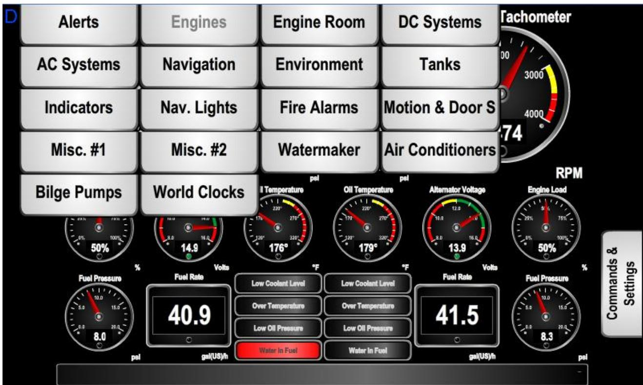
Figure 9 – N2KView® Window with Tabs Displayed
