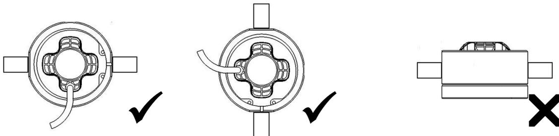
**Figure 1 - Correct and Incorrect Mounting Orientations**
