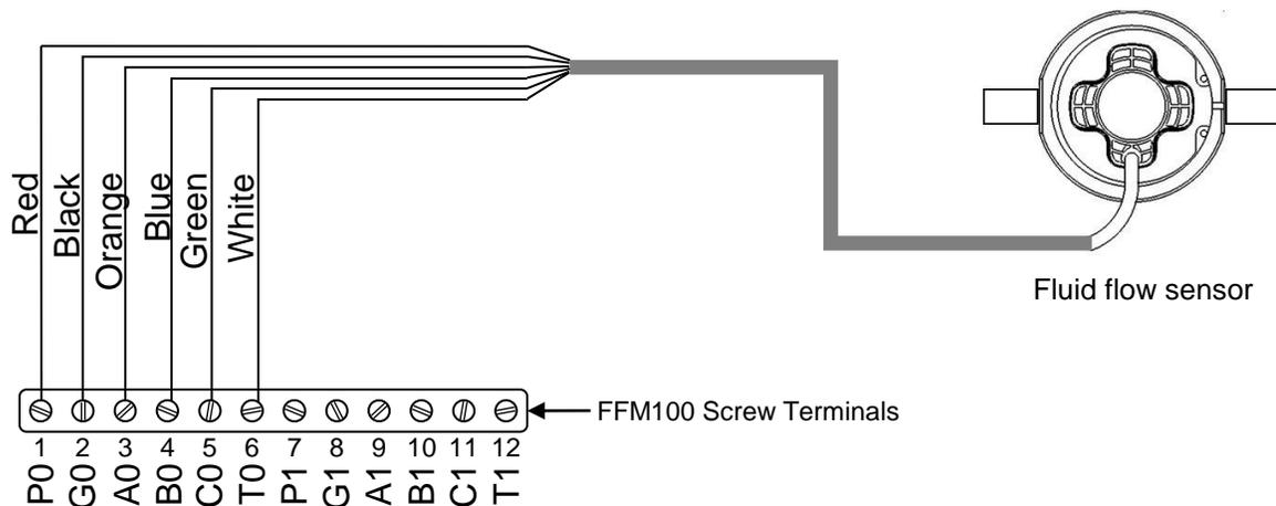
**Figure 2 - Fuel Flow Sensor Connection Diagram**
