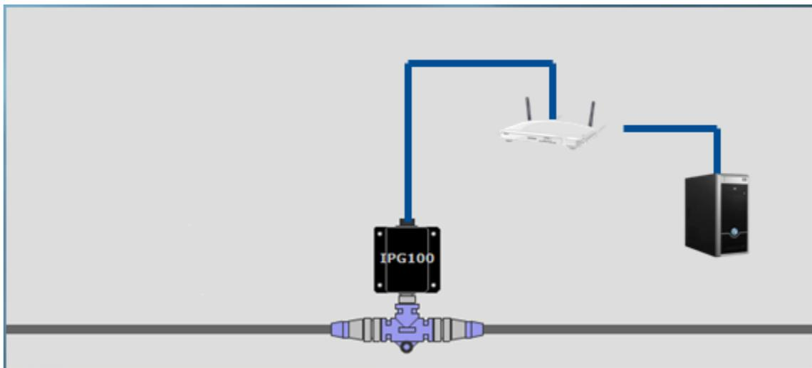
**Figure 4 – LAN Client/Server Architecture Example with IPG100**
