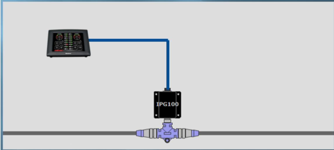
**Figure 5 – Single Client Connection to IPG100**
