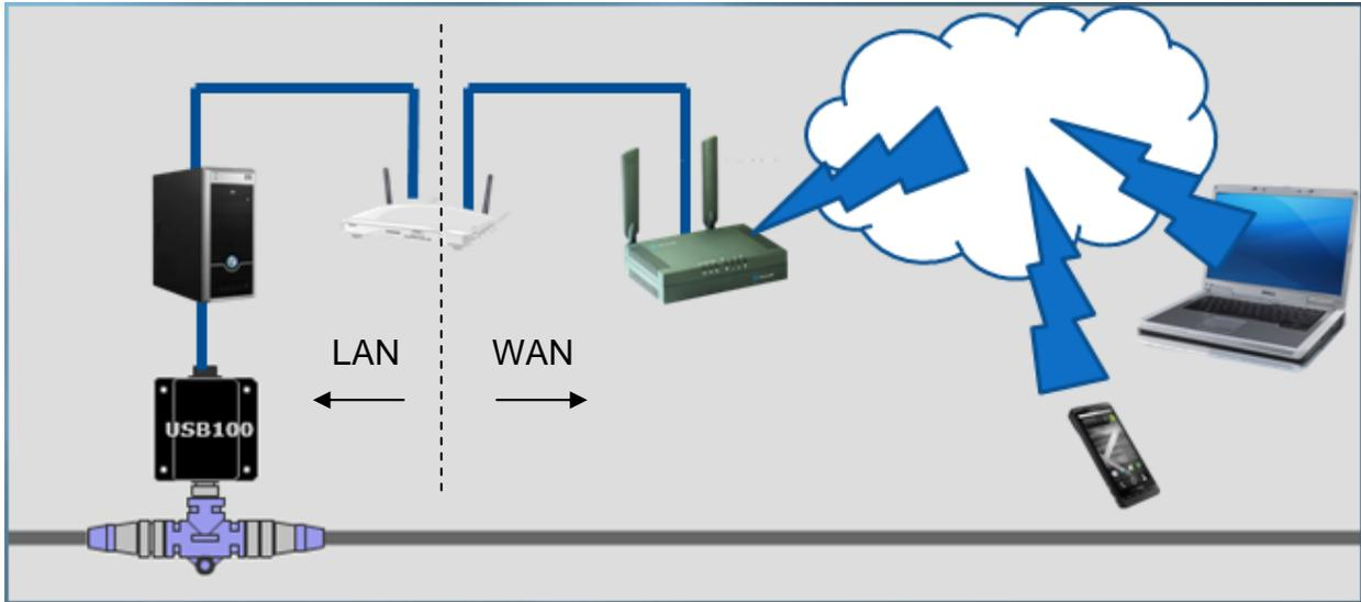
**Figure 3 – WAN Client/Server Architecture Example through the Internet**
