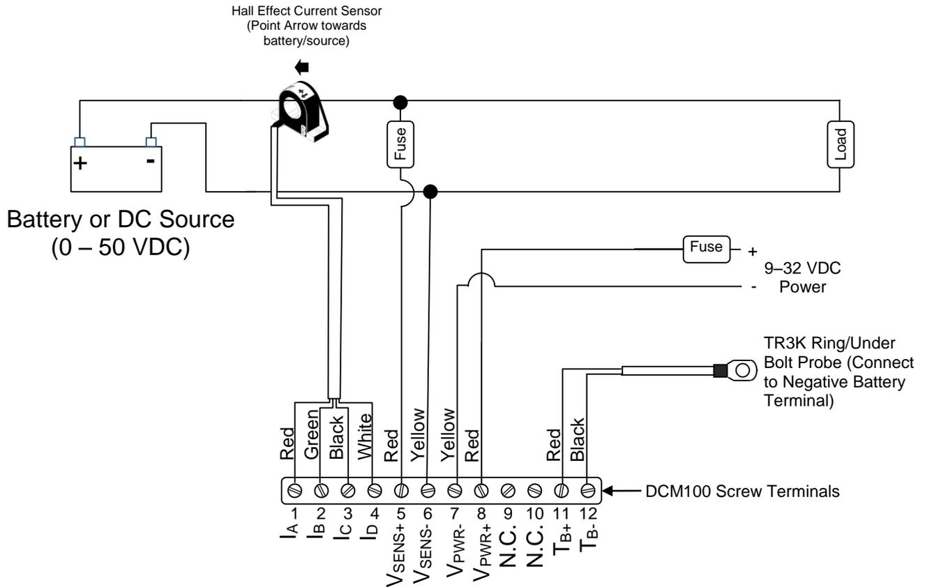
**Figure 3 – Connection Diagram**
